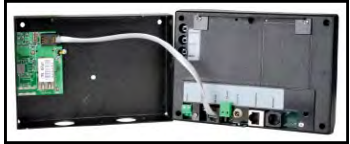
Figure 63. Connecting the Ethernet Board to the Smart Clock
