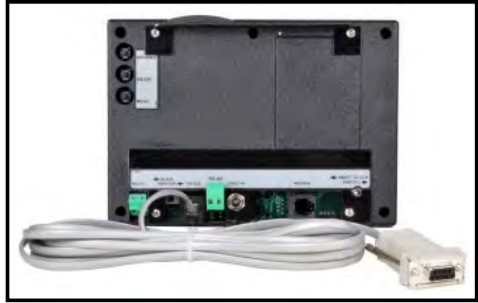
Figure 27. Connecting the telephone cord and RS-232 / Serial Port Adapter to the Smart Clock
