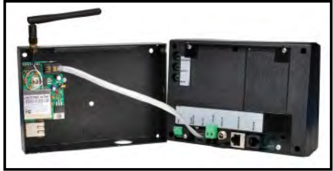
Figure 84. Connecting the Wireless Network Adapter to the Smart Clock
