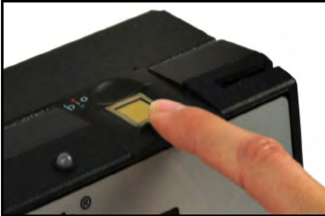
Figure 37. Touching the ridge-lock to discharge static electricity
