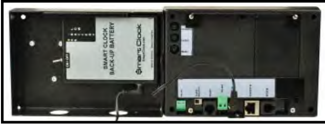
Figure 122. Connecting the Smart Clock Back-up Battery
